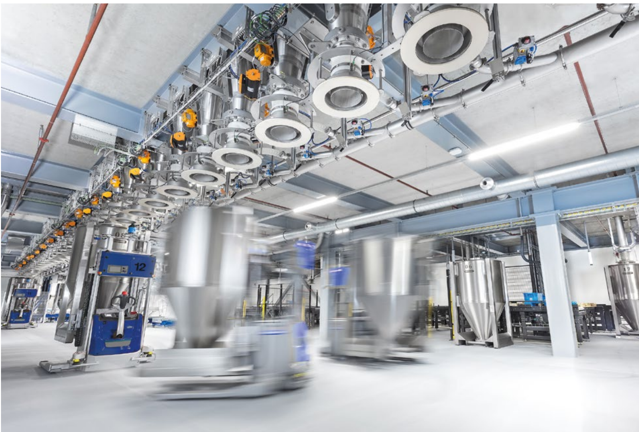
Fully automated collection system with Daxner Container System DCS combined with FTS System.
