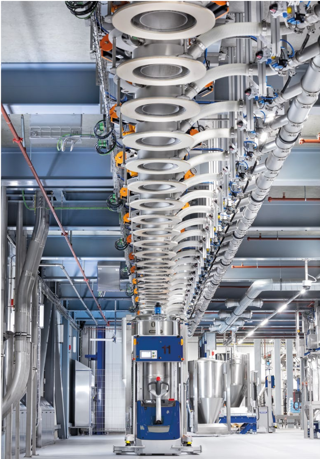
Fully automated collection system with Daxner Container Systems DCS in connection with the Automated Guided Vehicle system AGV.
